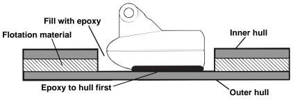
Epoxy the transducer to a solid portion of the hull.
